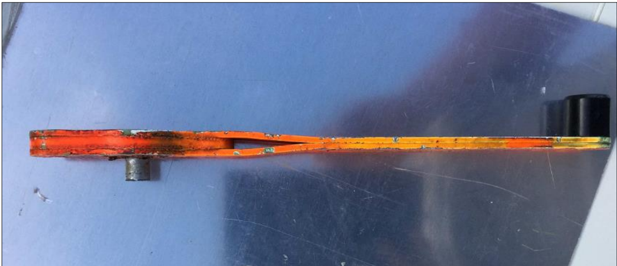
Figure 8: Broken Handle of the Emergency gear extension
