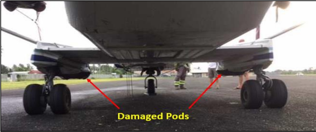
Figure 2: Damaged pods of the main landing gear
