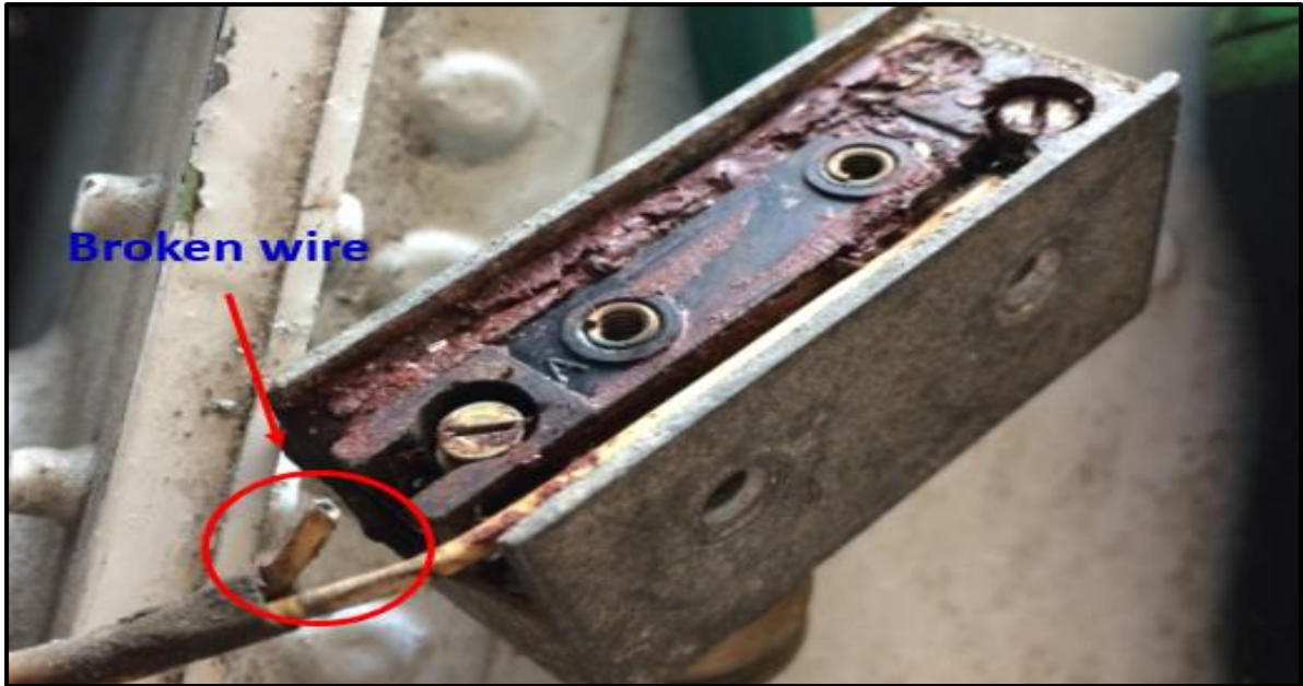
Figure 7: Broken Wire on the up-lock switch of the right landing gear
