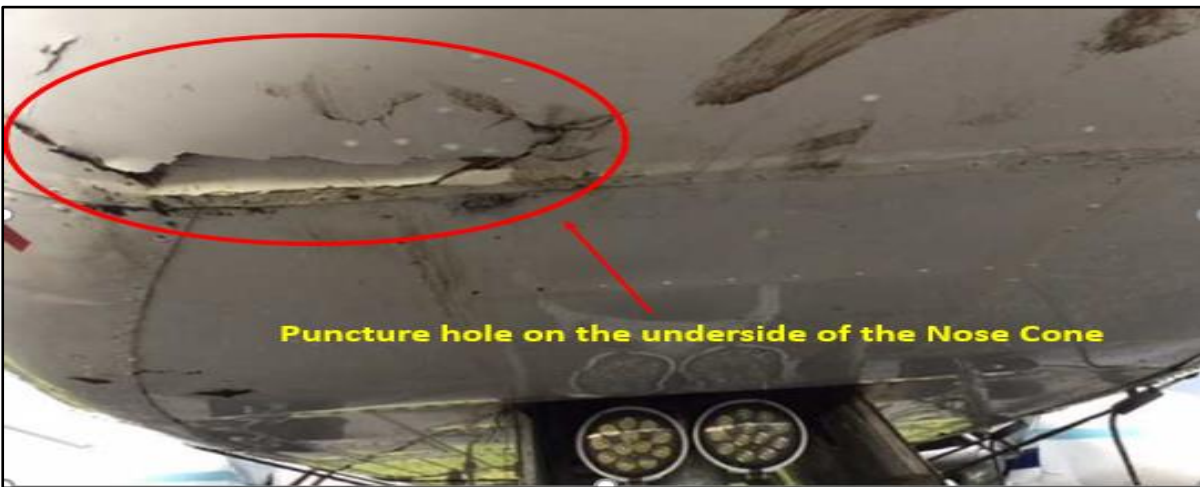
Figure 5: Puncture hole on the underside of the Nose Cone
