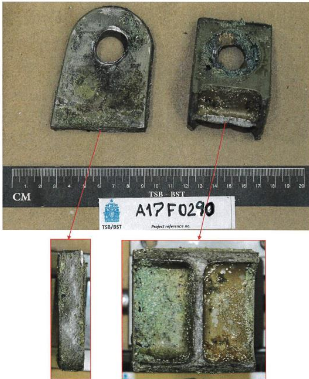
Figure 4: Separated pieces of the LH pylon to fuselage attachment (item 1b in Figure 1)
