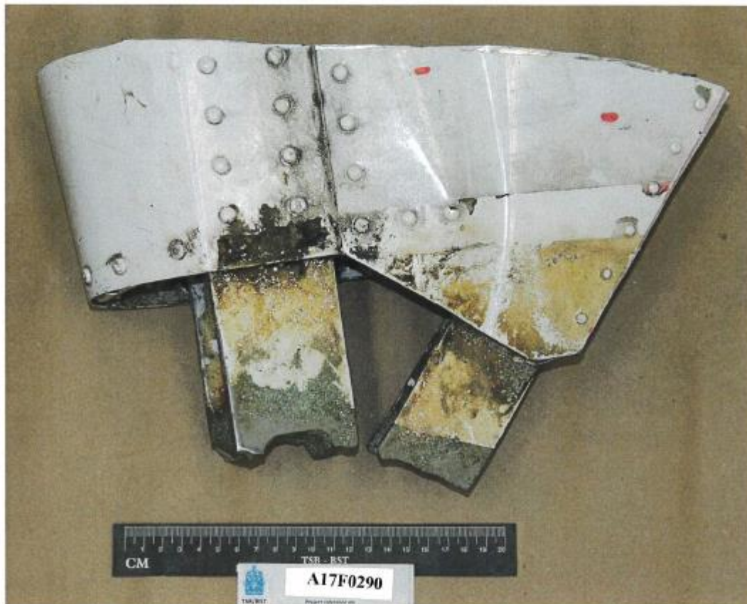
Figure 2: Cut-off piece of LH pylon to fuselage attachment (item 1a in Figure 1) photographed from the other side
