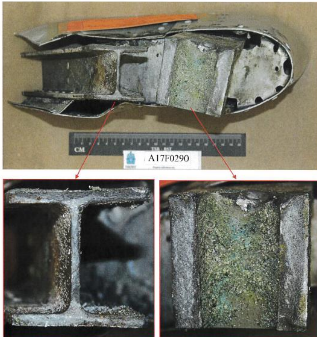
Figure 3: Cut-off piece of LH pylon to fuselage attachment (item 1a in Figure 1) photographed from the fractured side
