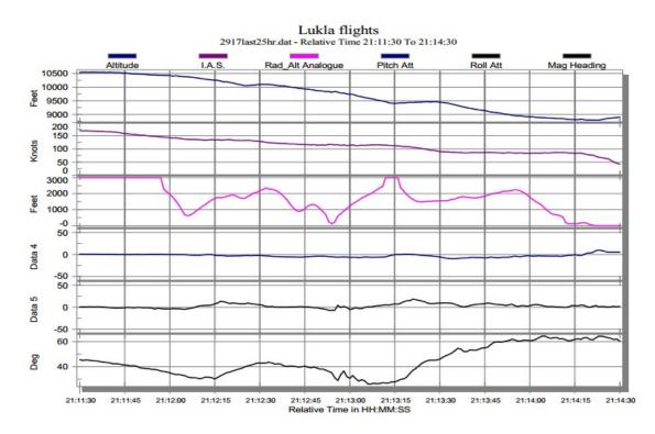
Figure 17: Last 3 minutes Data of 3<sup>rd</sup> flight to Lukla: at an interval of 15 seconds
