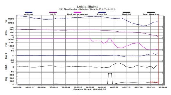
Figure 15: Last 3 minutes Data of 5<sup>th</sup> flight (crashed flight) : at an interval of 15 seconds
