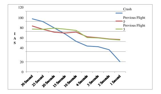
Figure 20: Comparison of Indicated air speed (IAS) among last three consecutive flights of 9N-AKY on 27<sup>th</sup> May 2017.
