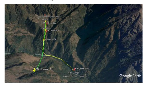
**Figure 22:**The track on the right-hand side was followed by ill-fated GOMA AIR aircraft 9N-AKY (commencing 60 seconds before impact). The track on the left-hand side is a hypothetical aircraft commencing normal approach to Lukla Airport.
