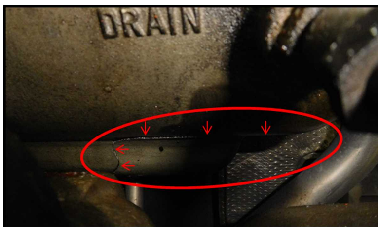
Photo #13-2. Cracks on the Fuel Oil Heat Exchanger
