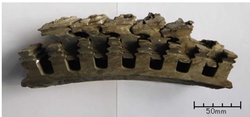
Photo #10. Piece of the 1st stage HPT disk rim
