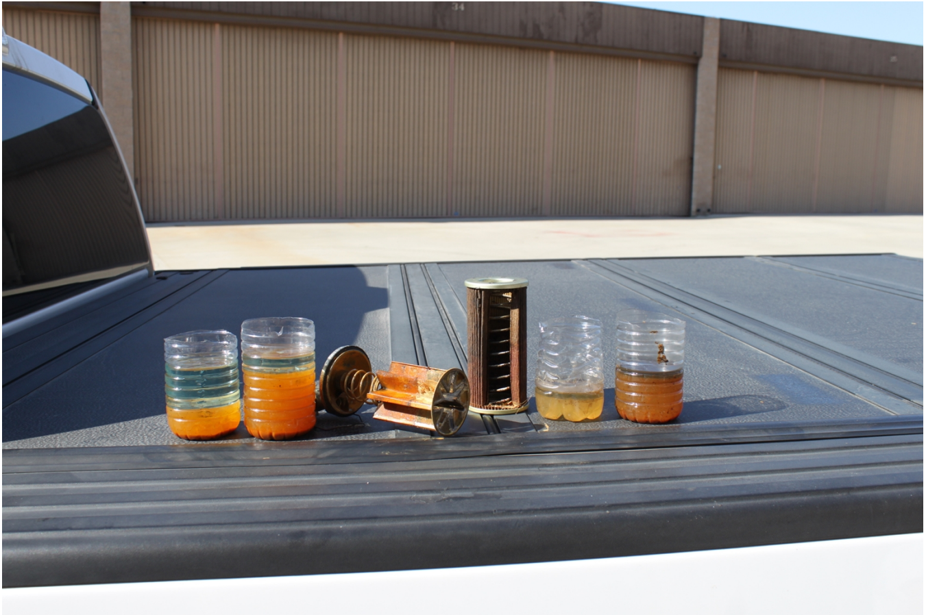
Photo 1 - Fuel and contamination removed from fuel lines and gascolator
