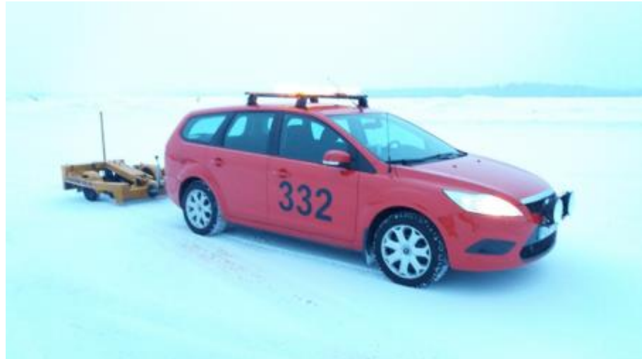
Figure 12. Vehicle with Skiddometer BV-11 (Photo: Lapland Airport).
