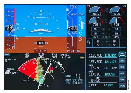
Figure 7: Primary Flight Display (PFD)
