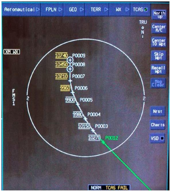
Figure 2. FMS Flight Plan/Waypoints Based on Data Provided
