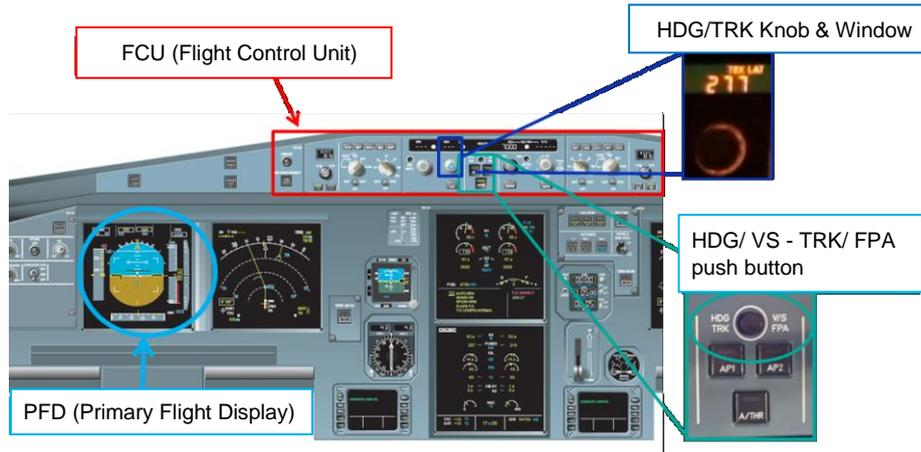
Figure 10: A320 Instrument Panels
