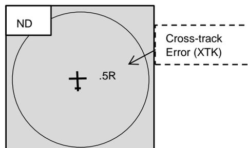
Figure 9: Deviation of horizontal direction (XTK)
