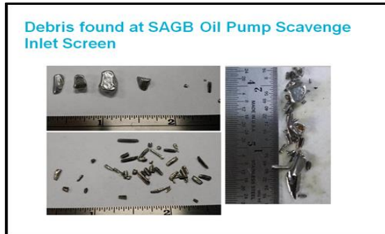
Figure 7. Debris from oil pump screen
