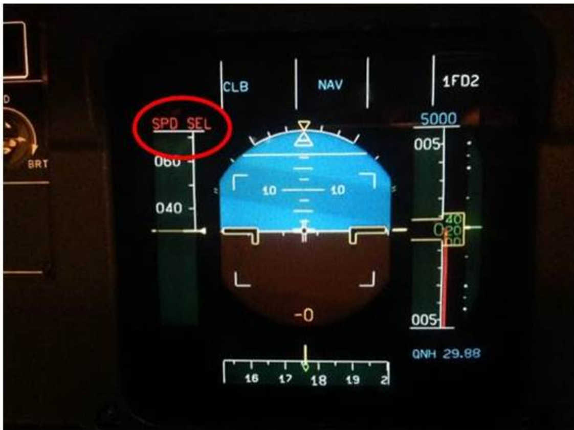
Figure 5. PFD after runway change with no V-speeds inserted in MCDU and SPD SEL on speed tape (indicated).
