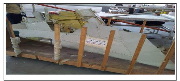
Figure 1.6B - Damaged Wing Tip
