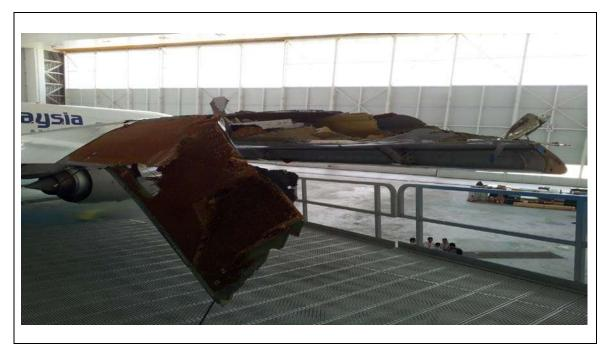
Figure 1.6A - Right Wing Tip Damage
