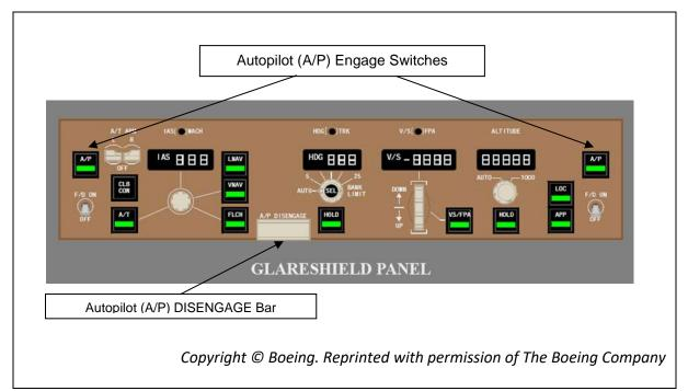
Figure 1.6C - Autopilot Mode Control Panel
