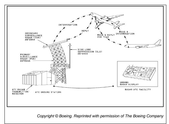
Figure 1.9A - Air Traffic Control/Mode S Transponder System
