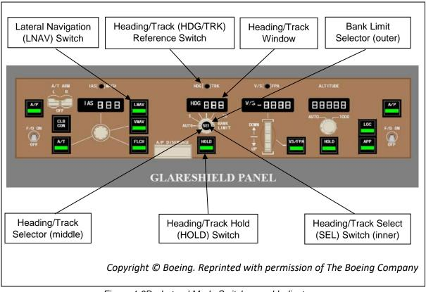
Figure 1.6D - Lateral Mode Switches and Indicators
