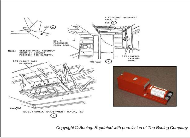
Figure 1.11A - Location of Solid State Flight Data Recorder
