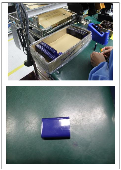
Figure 1.18E - Raw Single Cell Battery
