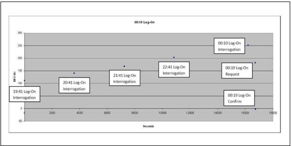
Figure 2.5D - Log-On Interrogation Transmissions
