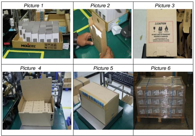
Figure 1.18H - Packing of Batteries by Motorola Solutions
