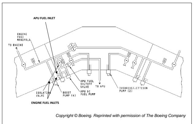
Figure 1.6I - Engine and APU Fuel Feed
