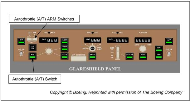
Figure 1.6G - Autothrottle Switches
