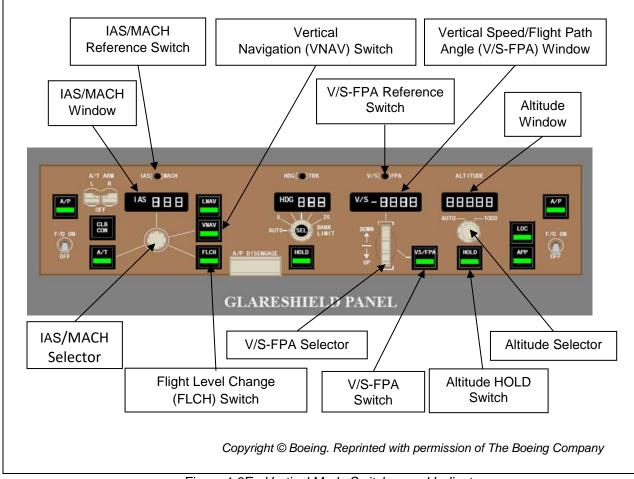
Figure 1.6E - Vertical Mode Switches and Indicators
