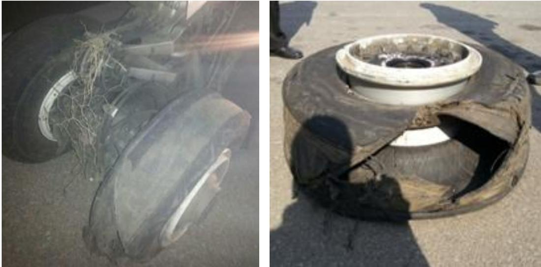
The aircraft had touched on the left side of the runway on soft ground. There was no damage to the aircraft on its first impact with the soft ground. The aircraft had rolled and then the left wheel had gone over the drain boundary area. The left main wheels got de-capped / damaged during this roll over/ skidding and during final stoppage with application of brakes.
