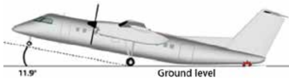
Figure 4. Fuselage strike, gear oleos extended
