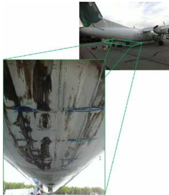
Photo 2. Damage observed under the fuselage (Source: Jazz Aviation LP)
