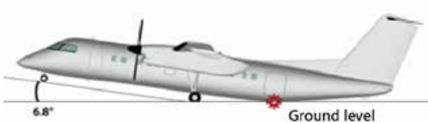
Figure 5. Fuselage strike, gear oleos compressed
