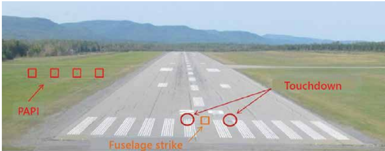
Photo 1. Touchdown point of the wheels and fuselage
