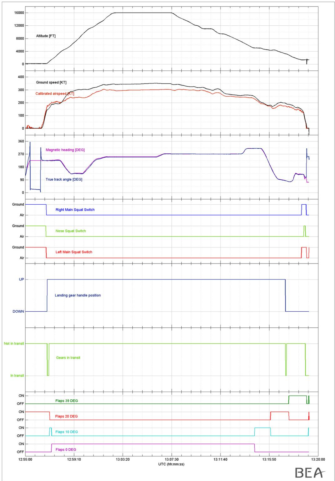
Figure 3: configuration of flaps and landing gear (complete flight)
