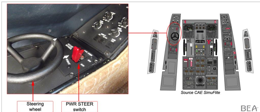
Figure 4: tiller and guarded PWR STEER switch
