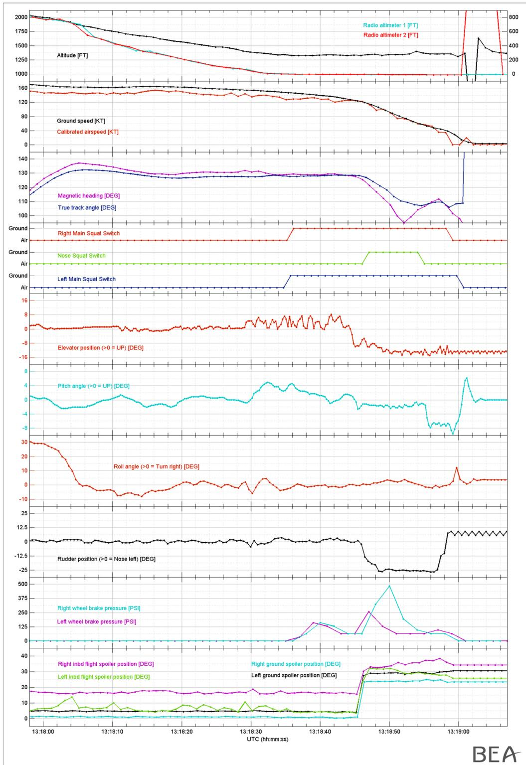
Figure 5: attitudes and position of aeroplane flight control surfaces (last minute)
