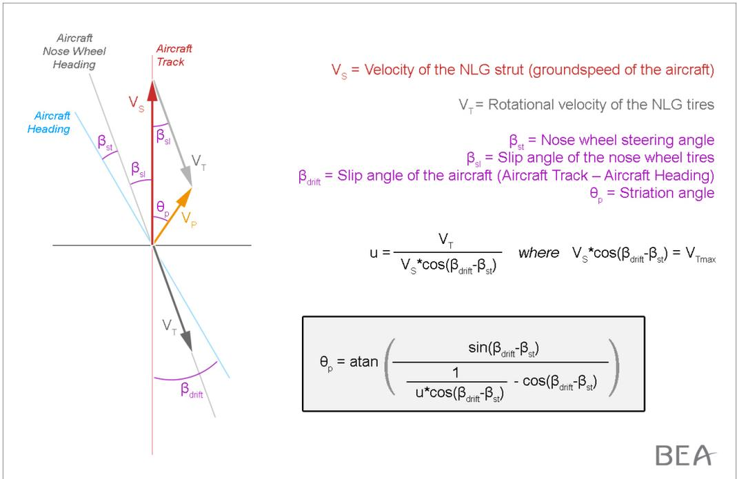
Figure 24: diagram of speed composition
