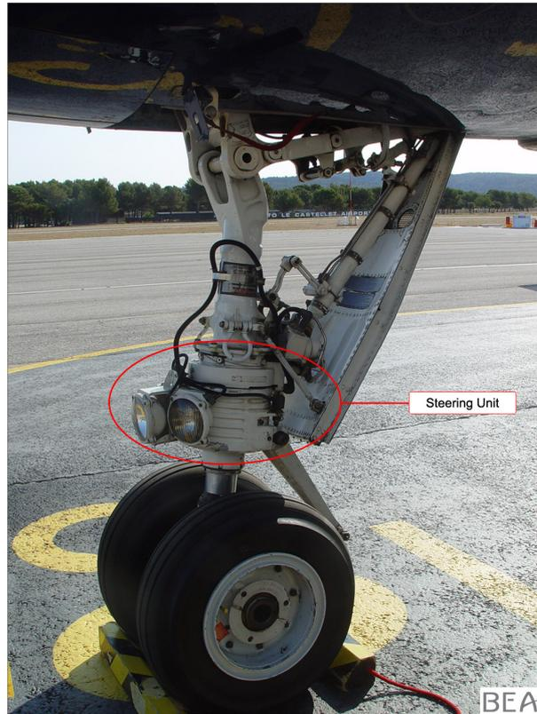
Figure 3: nose gear steering system of another G-IV
