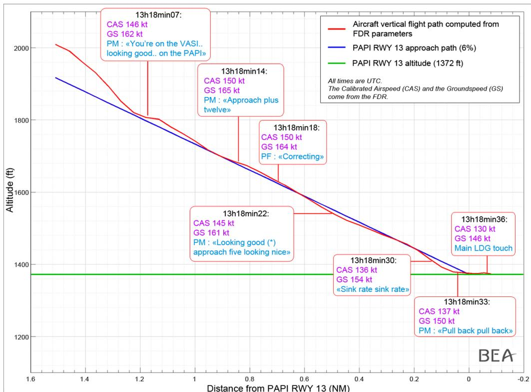
Figure 9: flight path in the vertical plane
