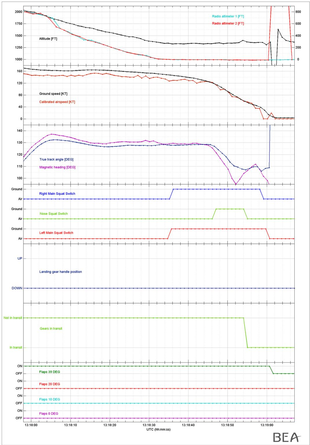
Figure 7: configuration of flaps and landing gear (last minute)
