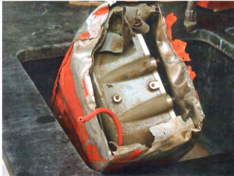
Figure 1. Damaged front end of flight recorder.
