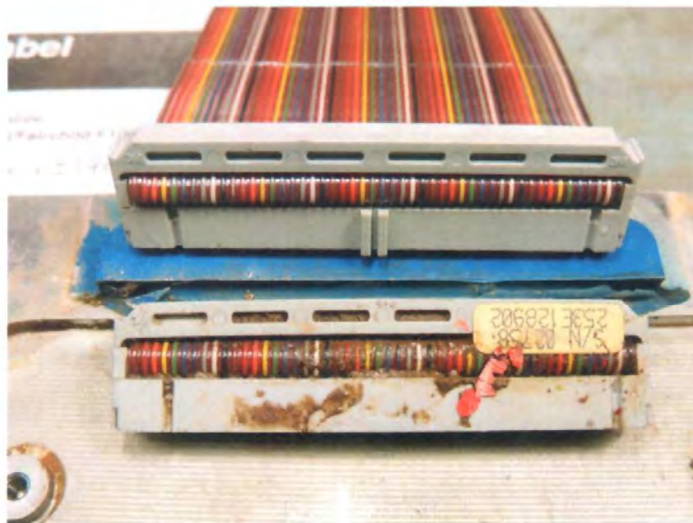
Figure 9. New connector crimped onto ribbon cable.
