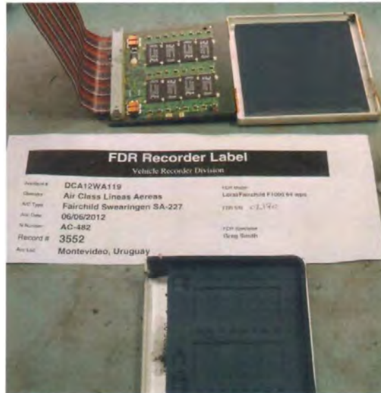
Figure 9. New connector crimped onto ribbon cable.
