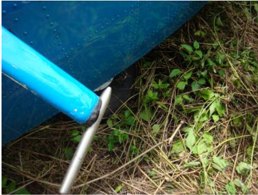
Figure 8: Nose landing gear collapsed backward to the left of fuselage
