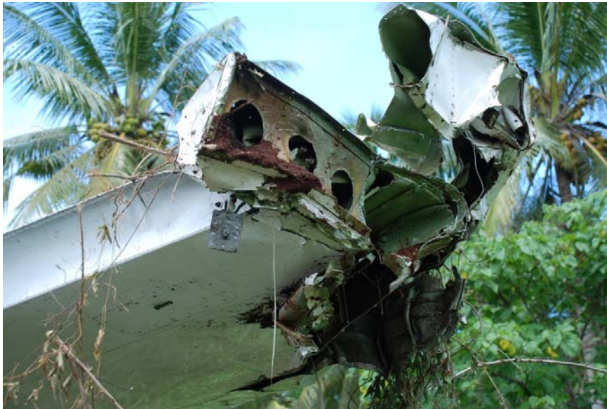
Figure 5. Right Wing Tip and right aileron were severe damage.
