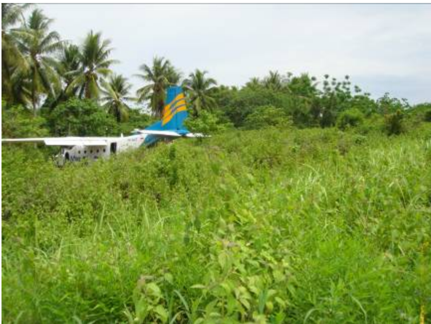
Figure 2: No sign of landing gears marking on the grass
