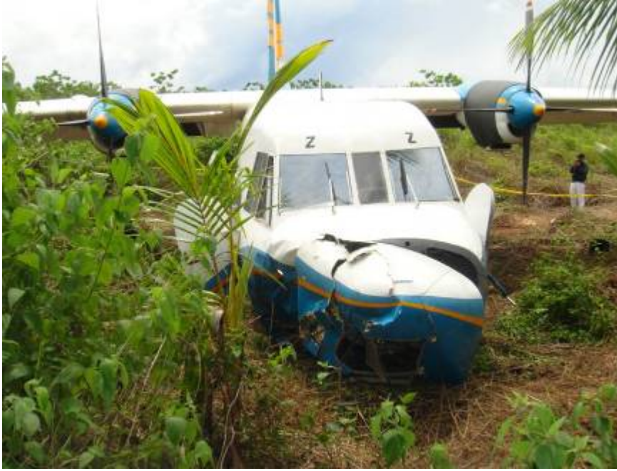
Figure 4: Nose section was severe damage
