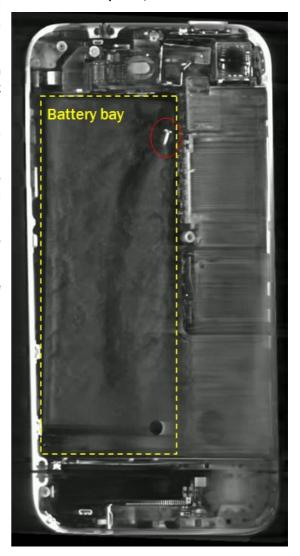
The completed examination concluded that the mobile telephone battery failure was most likely the result of the following sequence of events:
