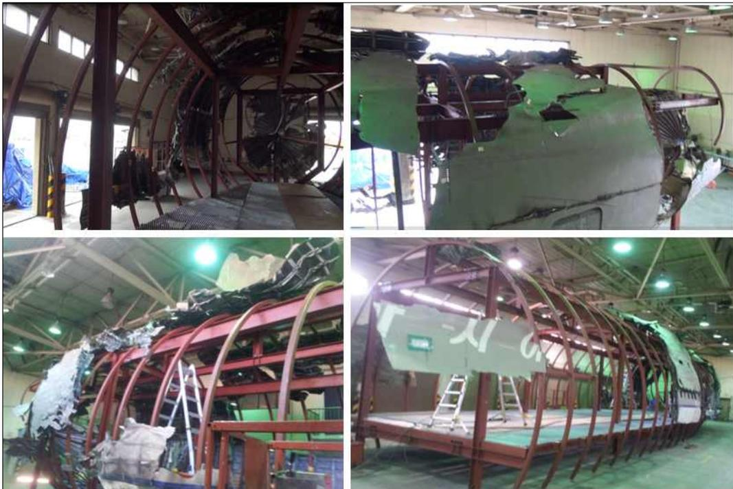
[Figure 45] Wreckage Reconstruction
