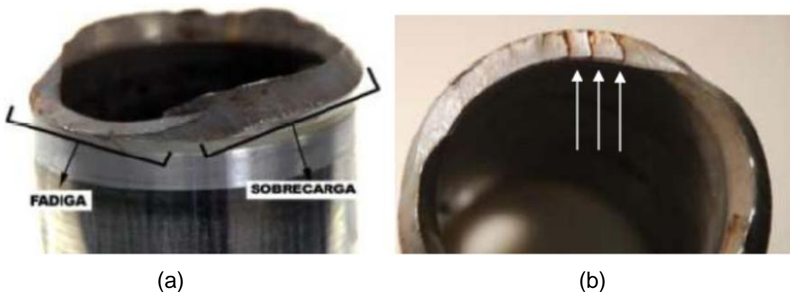
Figure 5 – Aspects of the pin (D61000 E1 SN 25). It is possible to see a flat fracture surface and another one at \pm 45^\circ (a). It is possible to observe multiple fracture plans, indicative of play, with various initiations (indicated by arrows) (b).
