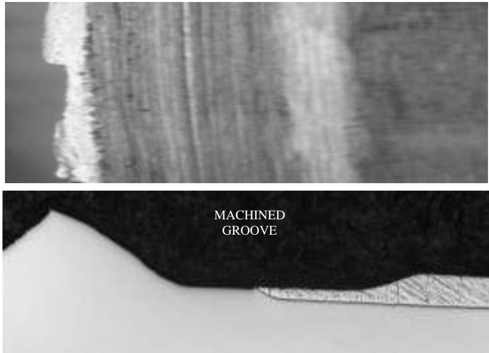
Figure 8 – Photographs showing the machined groove, and the area of the groove where the fatigue process occurred.
