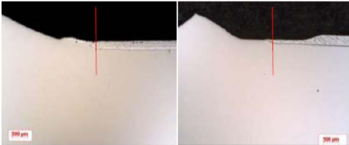
Figure 12 – Photomicrography. Comparison of the metallographic profiles between the pins D61000 MN 254 and D 61000 E1 SN 25, respectively, indicating that they were machined differently.
