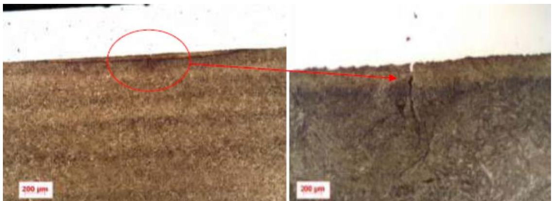
Figure 11 – Photomicrography. View of the section transversal to the crack, showing that the crack originated in a region that had sustained overheating.
