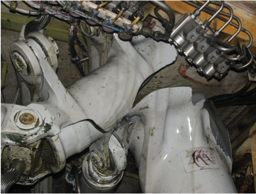
Abb. 1: Gebrochener Outer Cylinder
