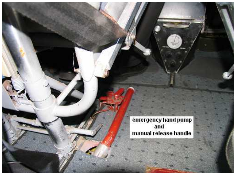
Figure 9 shows the emergency landing gear extension system.
