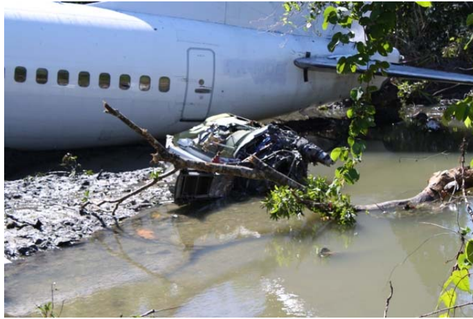
Figure 4: The left engine separated
