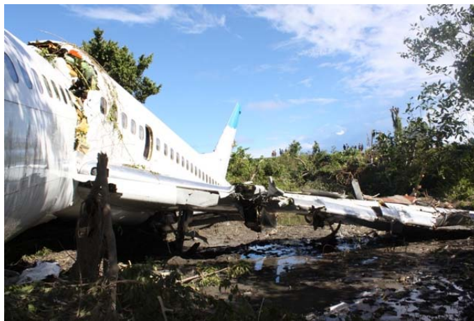
Figure 5: Left wing damage
