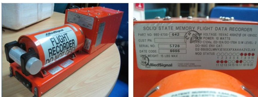
Figure 7: Flight data recorder
