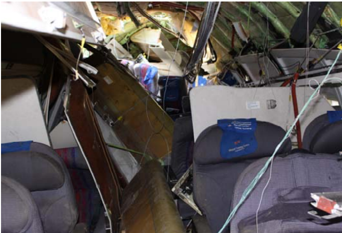
Figure 6: Passenger cabin damage
