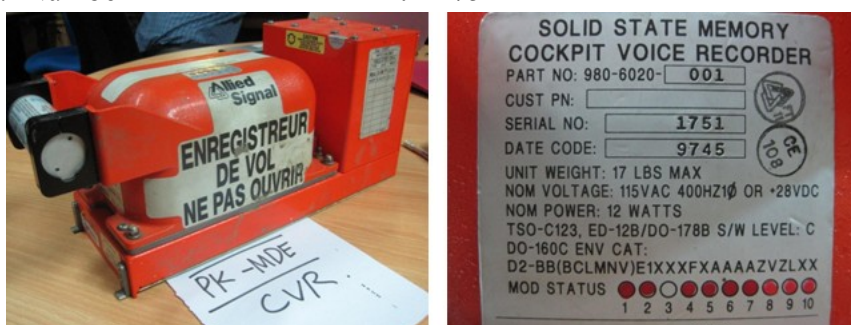
Figure 8: Cockpit voice recorder
