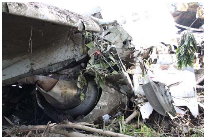
Figure 3: The right wing and number-two (right) engine damage
