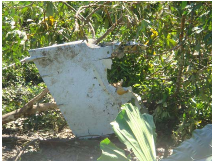
Figure 2: The left wing tip sheared off from the wing
