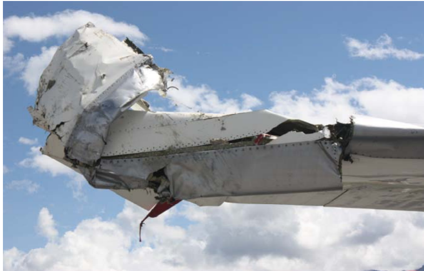
Figure 1: The damaged right wing tip
