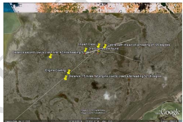
Figure 12 view showing location of 1st and 2nd cowling found in relations to the impact and debris field
