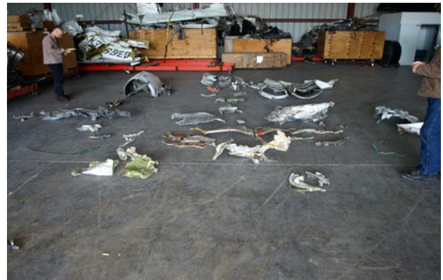
Figure 8 - Parts on the hanger floor represents the total recovered parts of the aircraft.
