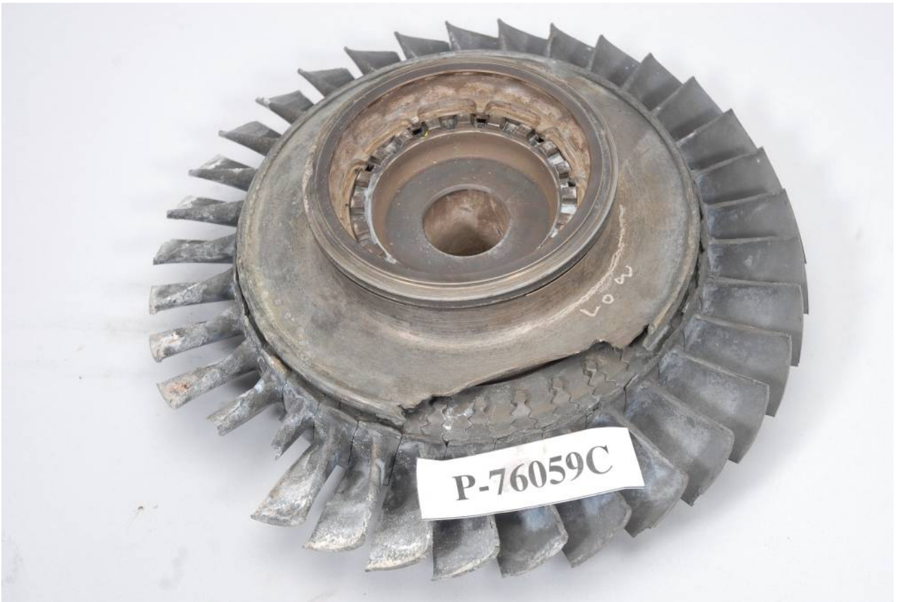
Figure 1. The failed seal plate.
