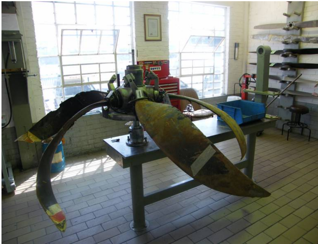
Figure 10. Damage to No. 2 propeller.
