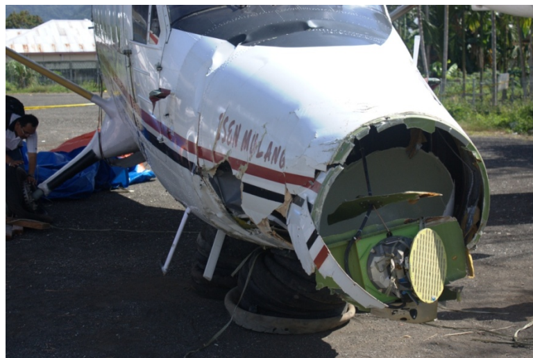
Figure 1: Damage on the nose section
