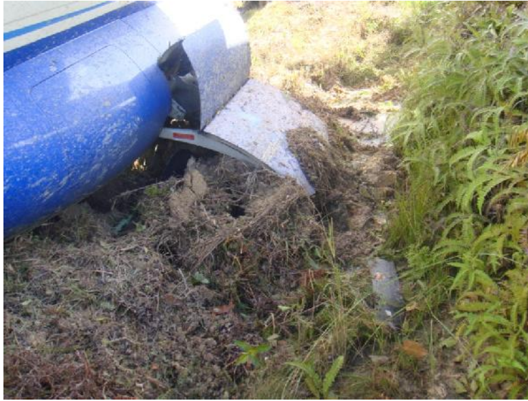
Figure 10: Propeller hit the mound, underneath the front of right gear
