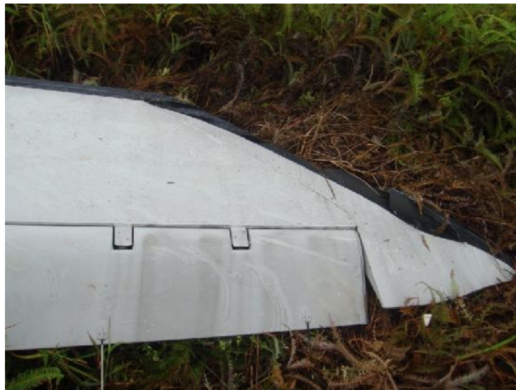
Figure 8: The right wing tip damage, no wrinkles on wing
