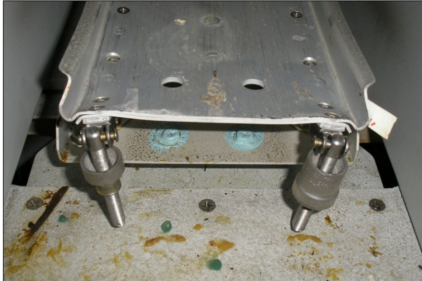
Figure A3: On-site photograph showing the original position of the threaded fasteners following the occurrence
