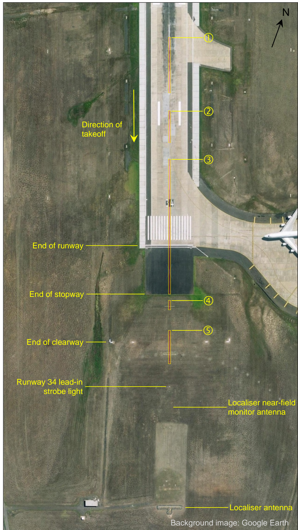
Figure 9: Ground contact marks
