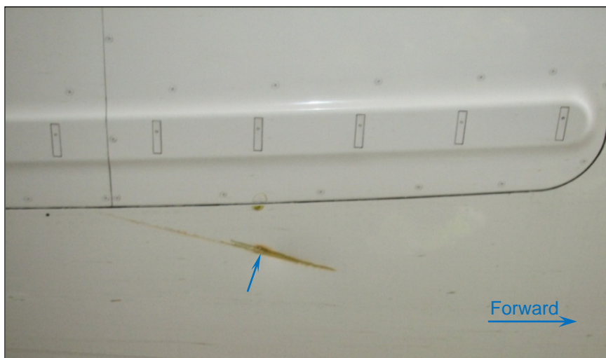
Figure 4: Contact mark below rear cargo door
