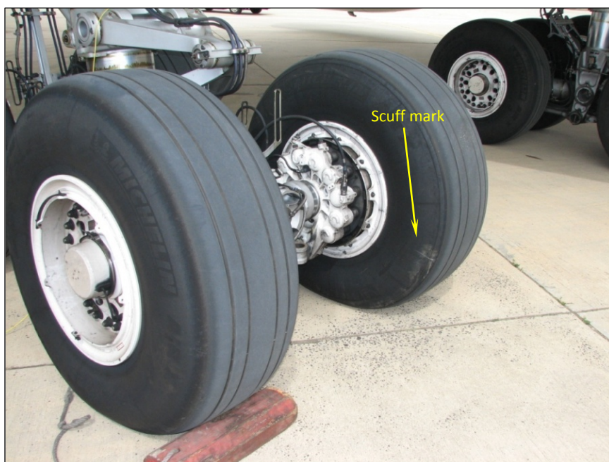
Figure 7: Contact mark on the left main landing gear, inboard rear tyre
