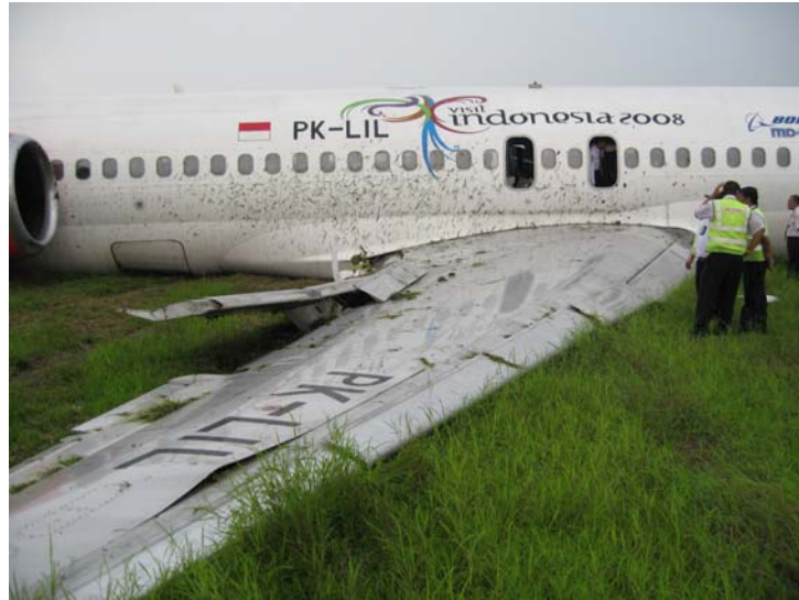
Figure 2: Right fuselage showing emergency exits opened, the damage of right wing and flap
