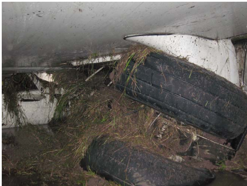
Figure 3: Left Main Landing Gear collapse sidewise
