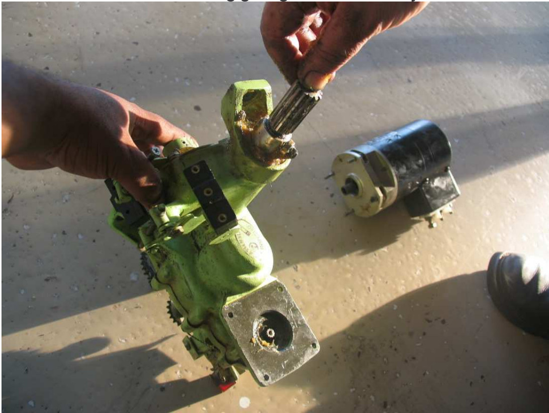
Photo 6: Illustrates the landing gear gearbox assembly and electrical motor.
