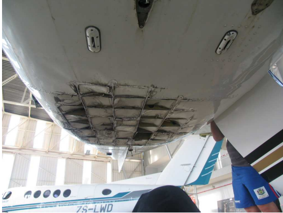
Photo 4: shows damage to port side inboard flap.
