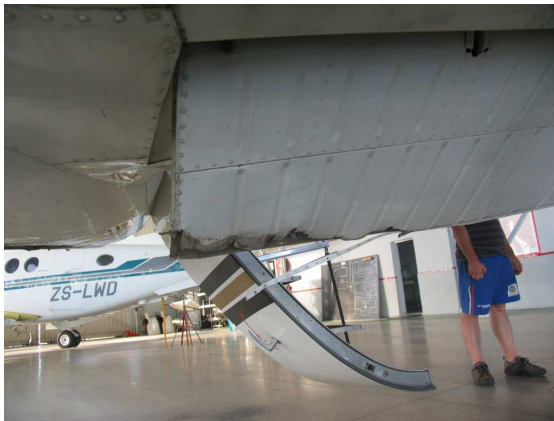
Photo 4: shows damage to port side inboard flap.
