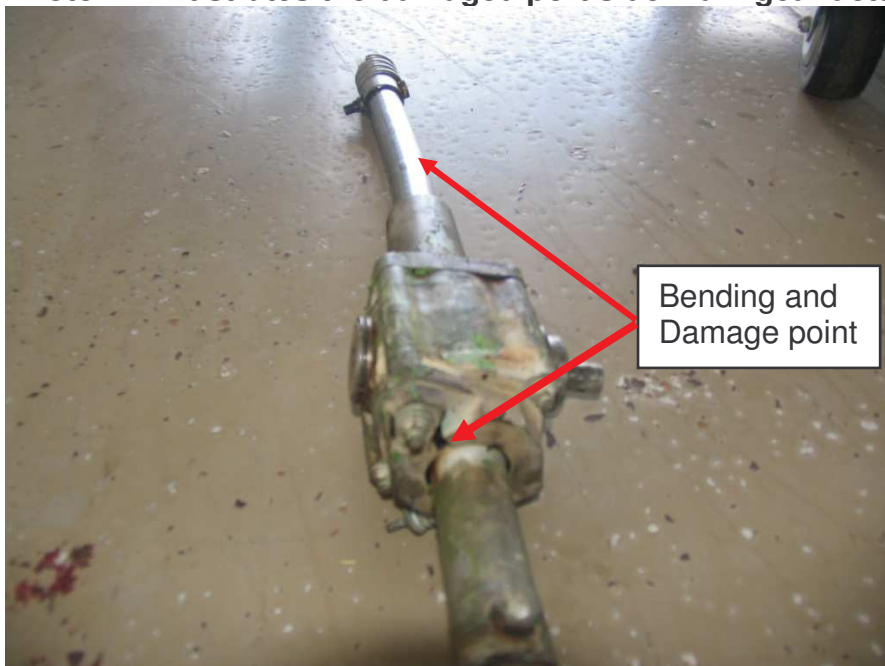
Photo 12: Illustrates the damaged port side main gear actuator.
