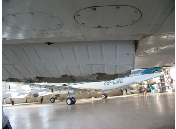
Photo 5 shows damage to the starboard main landing gear doors.
