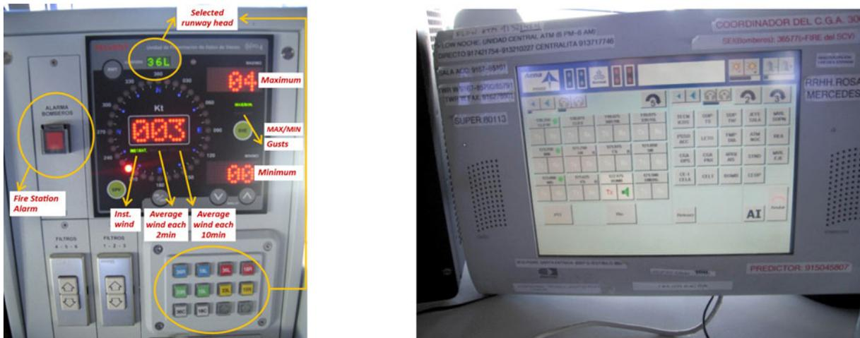
Figure 10. Wind monitor (zephyr) with the RFFS alarm and the scanner (CD30) at the Supervisor's positions
