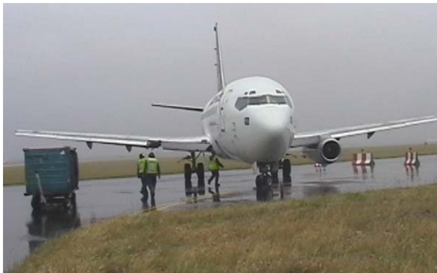
Photo 1: Showing the aircraft without the right-hand engine and parked on the taxiway.
