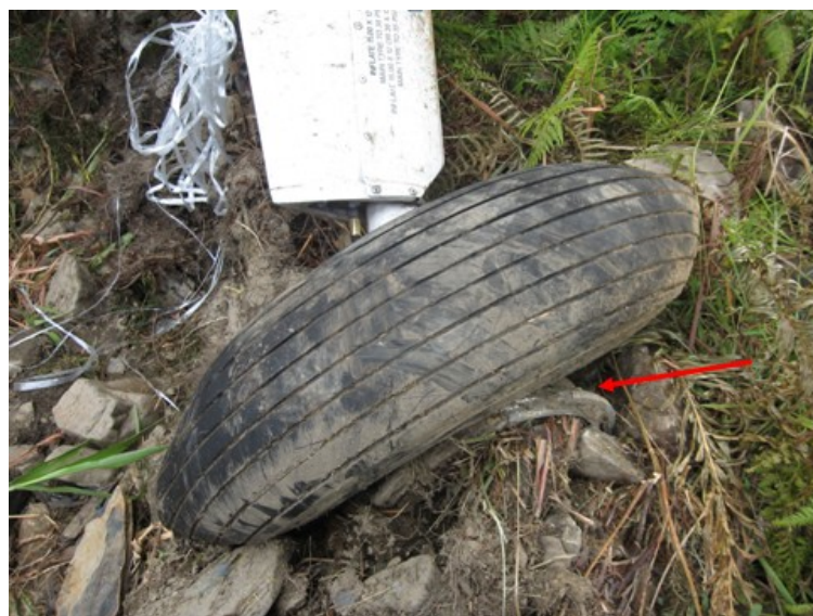
Figure 7 : The damaged right main landing gear wheel
