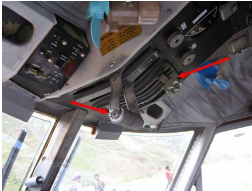
Figure 10 : Left arrow Power Levers and right arrow Propeller Levers
