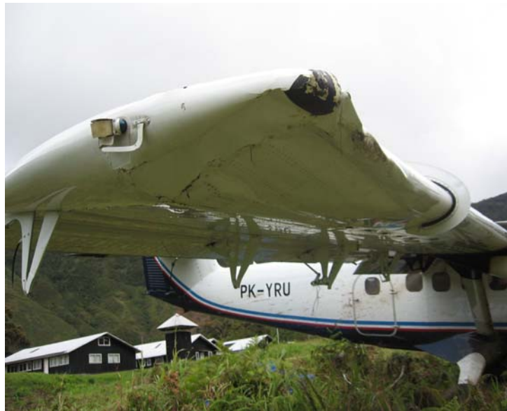
Figure 8 : Right wing substantially damaged
