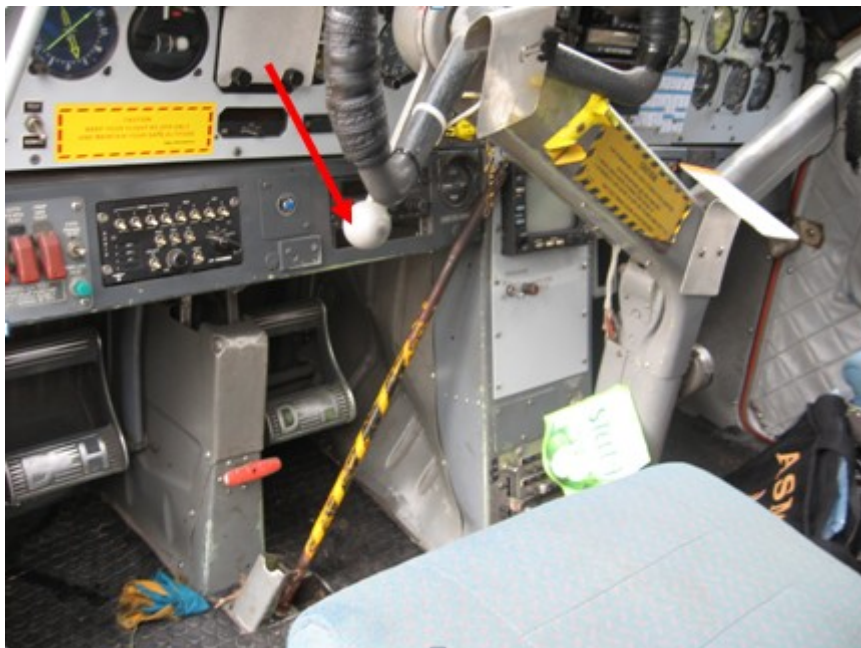
Figure 9 : Arrow pointing to the nose-wheel steering lever
