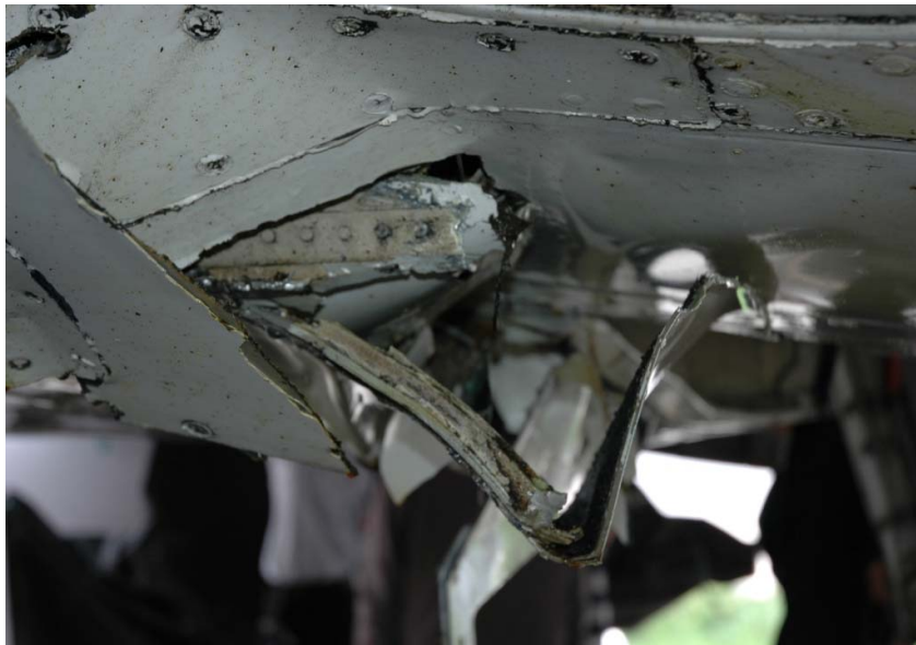
Figure 3: The Keel beam was broken
