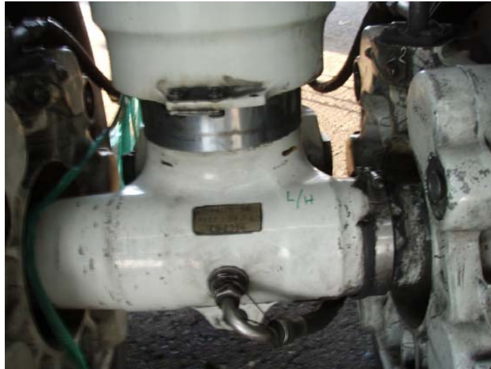
Figure 6: Bottoming marker on left main landing gear
