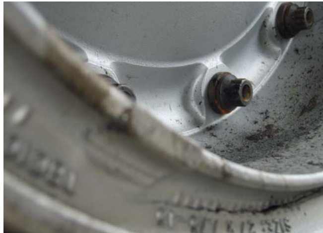
Figure 8: Wheel hub of the nose landing gear: crack
