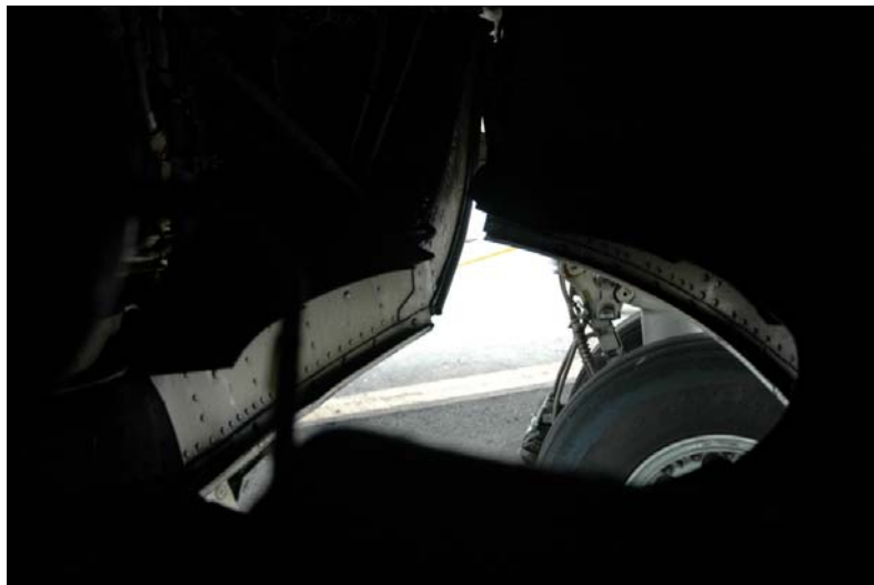
Figure 5: Wheel bay deformed
