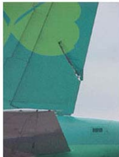
Damage Details between EI-CPE and G-BNLK
