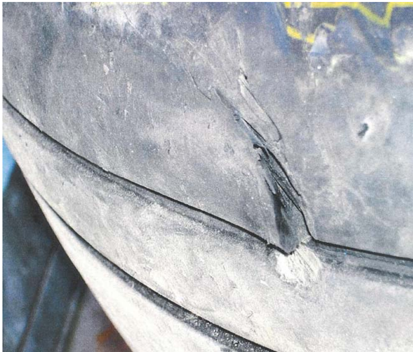
Damaged aircraft tires
