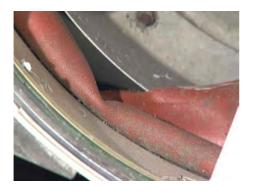
Figure 146: Diaphragm, showing typical tear.
