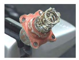
$\underline{\mbox{Figure 255:}}$  Integral sensor spring and diaphragm.
