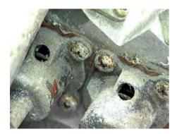
Figure 241: Cabin pressure sense ports.
