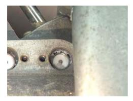
Figure 256: Opposite end of integral sensor poppet and guide; heavy salt deposits.
