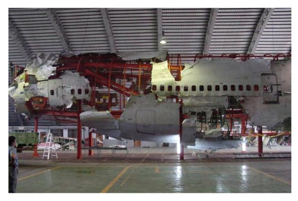
Figure 1.19-3 3D hardware reconstruction (right side)
