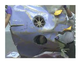
Figure 5: Pressure Relief Valves
