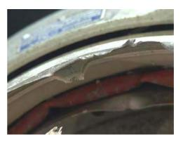
Figure 223: Knife-edge damage.
