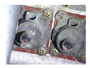
Figure 159: Control adjustment screws.
