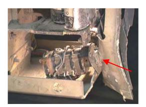
Figure 10: MODE SELECT Rotary Switch
