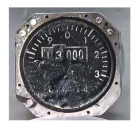
Figure 43: Cabin Altimeter Indicator, glass bezel removed
