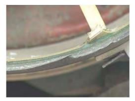
Figure 140: Close-up of knife-edge damage.
