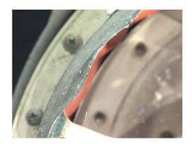
Figure 139: Close-up of knife-edge damage.
