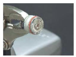
$\underline{\mbox{Figure 253:}}$  Plug HS P/N 719280-1 and seal, seal looks normal and uncut.
