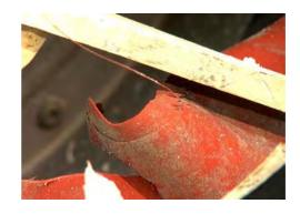
Figure 227: Outer diaphragm HS P/N 727403-1, torn location.
