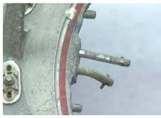
$\underline{\mbox{Figure 106:}}$  Aft hinge & stop pins (looking from inside to outside).
