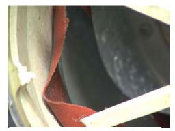
Figure 230: Outer diaphragm damage.
