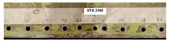
Figure 1.16-6 Light colored deposit on the faying surface of the repair
