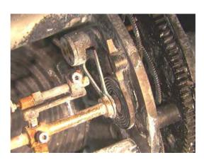
Figure 46: Cabin Altimeter Indicator, bellows, visible damage
