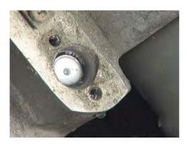
Figure 169: Shows water in plug area.
