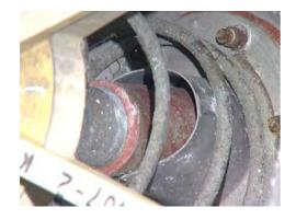
$\underline{\mbox{Figure 153:}}$  Center diaphragm & return spring.
