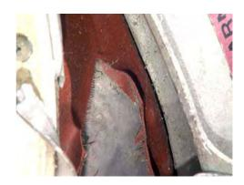
$\underline{\mbox{Figure 233:}}$  Outer diaphragm, close-up of tear origin.
