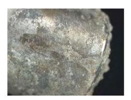
$\underline{\text{Figure 124:}}$  Aft/upper stop pin, close up of figures #122 & #123, after pin was cleaned with alcohol.
