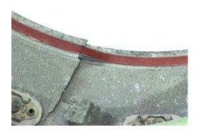
Figure 99: Another cut on the seal.
