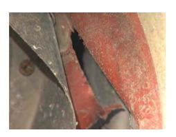
$\underline{\mbox{Figure 228:}}$  Outer diaphragm, approximately 60% of circumference is torn.
