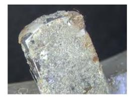
$\underline{\underline{Figure~120:}}$  Forward/upper stop pin, close-up of figure #119.
