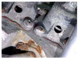
$\underline{\mbox{Figure 158}}:$  Cabin pressure sense ports on sensor adjustment springs.
