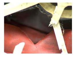
Figure 229: Outer diaphragm, torn location.
