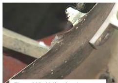
Figure 225: Knife-edge damage.
