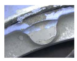
Figure 191: Upper stop pad; paint chipped.
