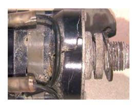
Figure 30: Switch #3 body crack detail
