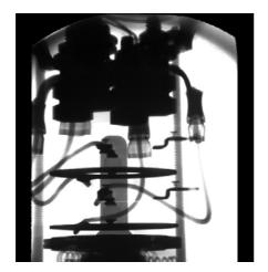
Figure 35: X-ray of Bleed Air Valve Switch #2.
