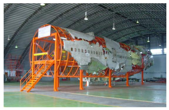
Figure 1.19-4 3D hardware reconstruction
