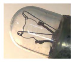
Figure 39: **PRESS RELIEF** light, upper right lamp, (filament intact). - (Ref. Figure 37, yellow arrow for lamp location).
