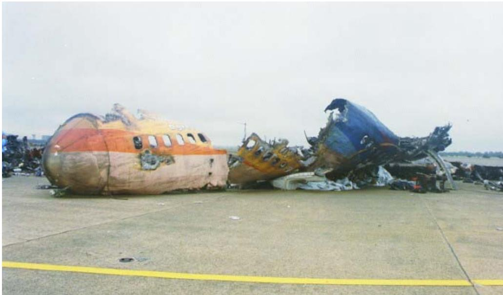
**Figure 1.12-6 Front portion of the aircraft**
