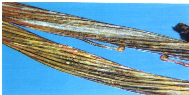
**Figure 1.16-7 RE240-1, localized melting near the boundary of insulation that was lost.**
