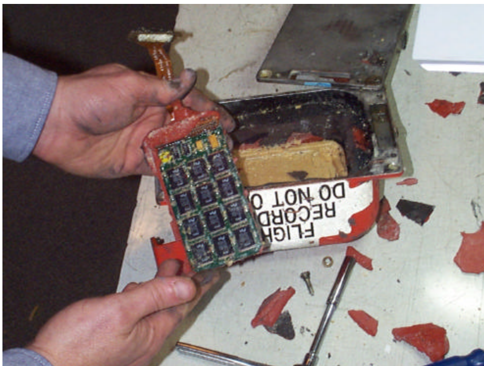
Figure 5.b Memory module of the Solid State CVR
