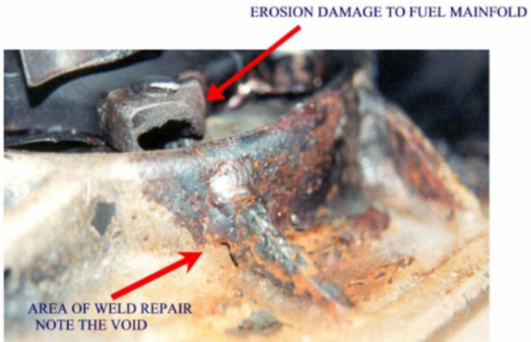
PHOTOGRAPH OF THE INTERIOR OF THE DIFFUSER CASE SHOWING THE P&D VALVE MOUNTING-BOSS & DETAILING THE EROSION DAMAGE TO THE FUEL MANIFOLD AND THE DEFECTIVE WELD REPAIR
