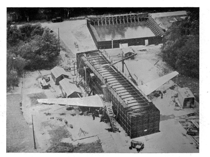
FIG. 6. AERIAL VIEW OF COMET G-ALYU IN TESTING TANK.
