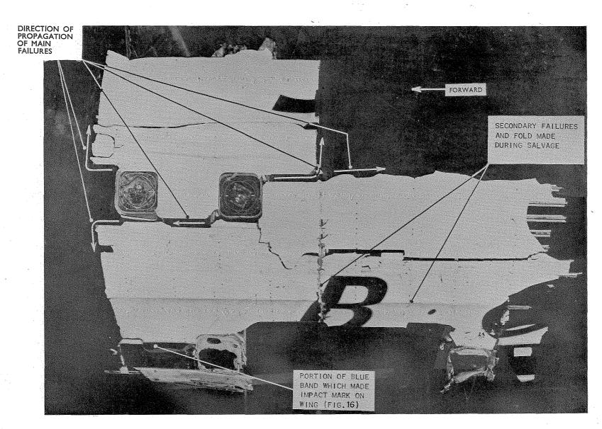
FIG. 12. PHOTOGRAPH OF WRECKAGE AROUND ADF AERIAL WINDOWS-G-ALYP.
