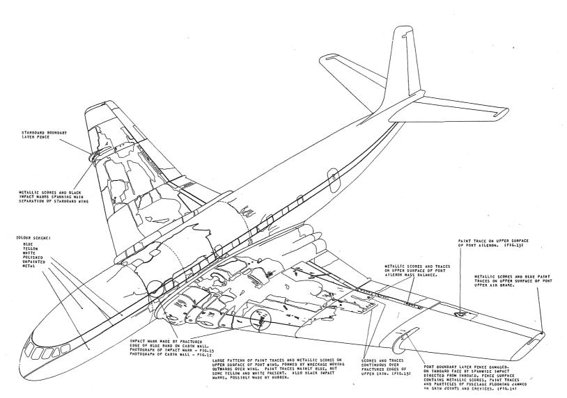
FIG. 16. IMPACT DAMAGE TO UPPER SURFACES OF WINGS-G-ALYP.
