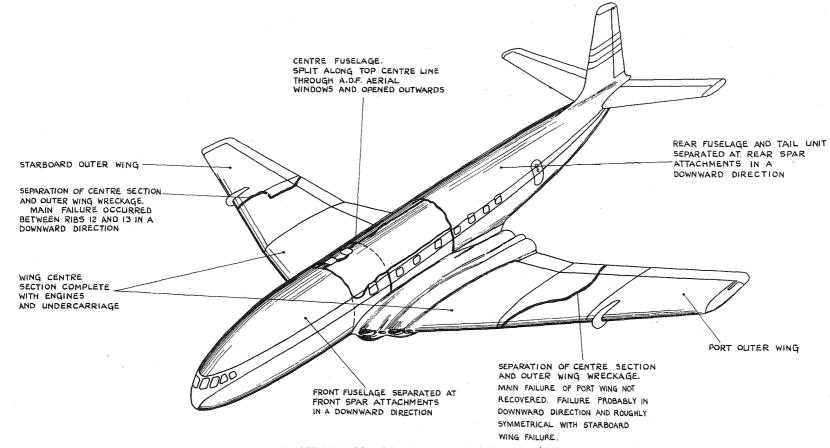
FIG. 11. LOCATION AND DIRECTION OF MAIN FAILURES-G-ALYP.
