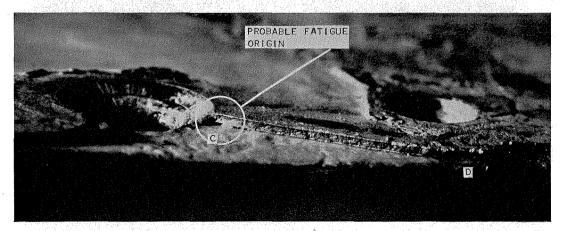
(c) VIEW OF EDGE C D. FIG. 19. SIGNS OF FATIGUE IN SKIN AT STARBOARD REAR CORNER OF REAR ADF AERIAL WINDOW-G-ALYP.
