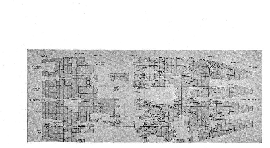
FIG. 3. DEVELOPMENT DRAWING OF FUSELAGE SHOWING AMOUNT OF WRECKAGE RECOVERED-G-ALYP.
