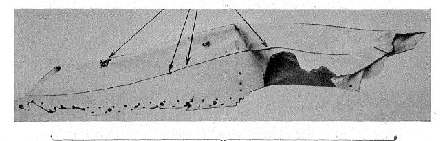
GENERAL PATTERN OF METALLIC SCORES AND PAINT TRACES OVER INBOARD FACE PROGRESSING FROM WING SKIN TO UPPER EDGE OF FENCE
