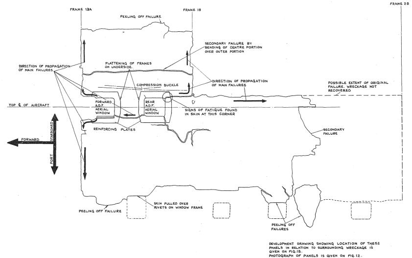
FIG. 17. SALIENT FEATURES OF DISRUPTION OF PRESSURE CABIN-G-ALYP.
