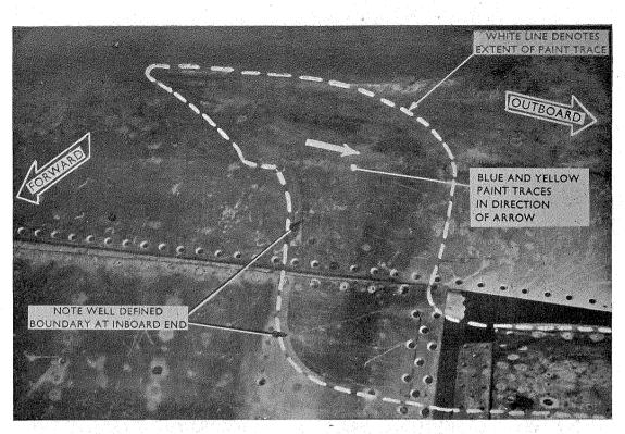
PAINT TRACES MADE BY PORTION OF CABIN WALL (FOR LOCATION SEE FIG. 16).
