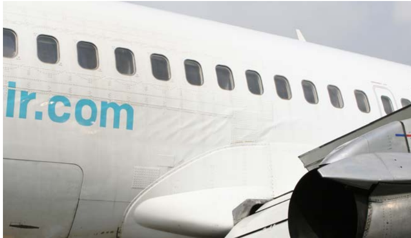
Figure 2: Wrinkling on the right centre fuselage section
