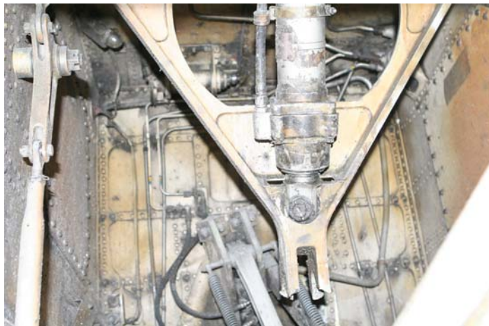
Figure 1: Fractured lower strut of the nose landing gear
