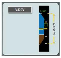
Note: According to DFDR, the L/DEV and V/DEV information was displayed on both PFDs during the approach (Ref. DFDR parameters "CLATDEVD", "CVERTDEVD" for the captain's PFD and "FLATDEVD" and "FVERTDEVD" for the F/O's PFD).
