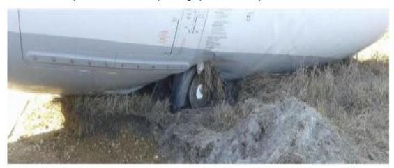
Inlet, fan and reverse cowls were sheared off on both Engines:
